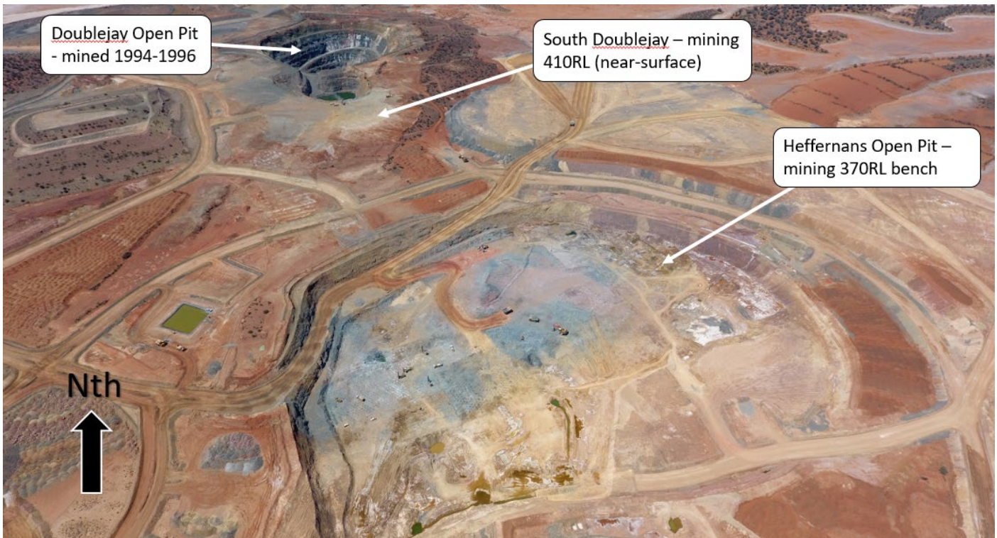
Figure 2: Aerial photograph of current mining activities at Jupiter showing Heffernans mining on the 370RL bench and South Doublejay commencing mining operations at the 410RL. Ganymede has also commenced mining south of the Heffernans open pit.
