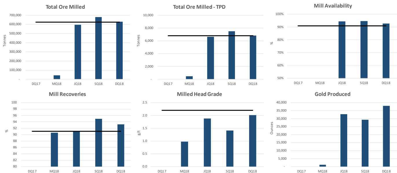
Figure 5: Summary of the key operating performance measures of the MMGO processing plant from first gold in late March 2018. Note performance levels for the majority of the measures are at or above Feasibility design levels (i.e. steady state) depicted by the horizontal black lines on the charts]
