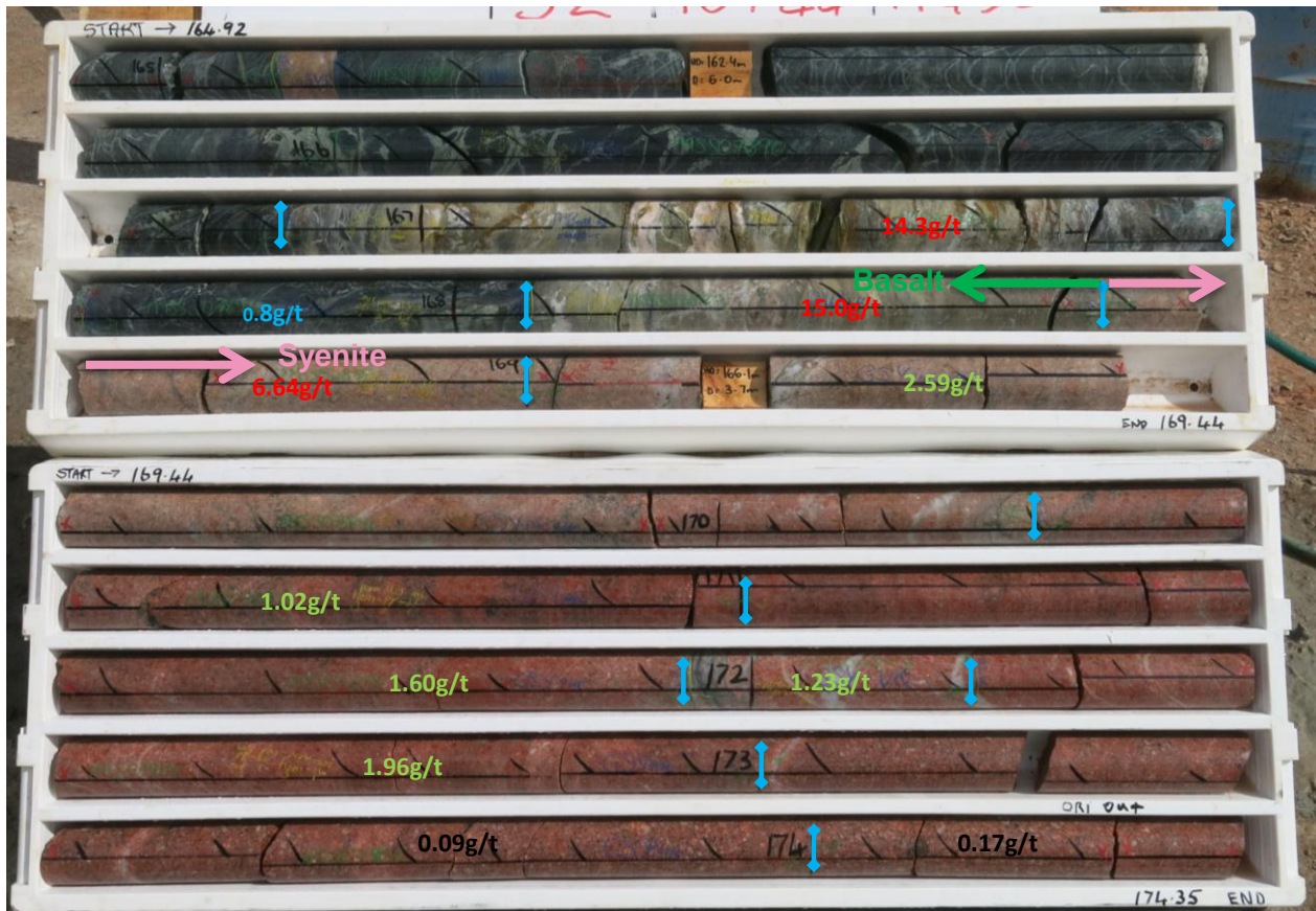
Figure 4: Core photographs and assay values for intersection of 6.12m @ 4.8g/t in 13JURD006 showing high grade gold defined adjacent to the contact of the syenite (See Figure 3 for cross section reference)
