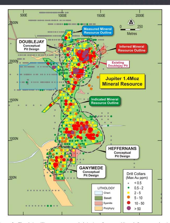
**Figure 1**: The 1.4 million ounce upgraded Jupiter Prospect Mineral Resource showing conceptual open pit outlines, drill density with maximum grade intersected; and resource classification outlines.
