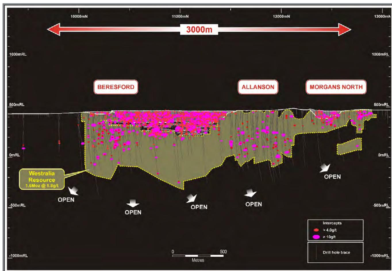
**Figure 3:** Longitudinal section of the 3km long Westralia Deposit Mineral Resource (yellow shading) showing the location of the recently completed 24 hole, 11,000m in-fill diamond drilling program at Beresford and the 71 hole, 35,000m in-fill drilling program at Allanson. Note the high proportion of +10g/t Au intersections from both drilling programs.
