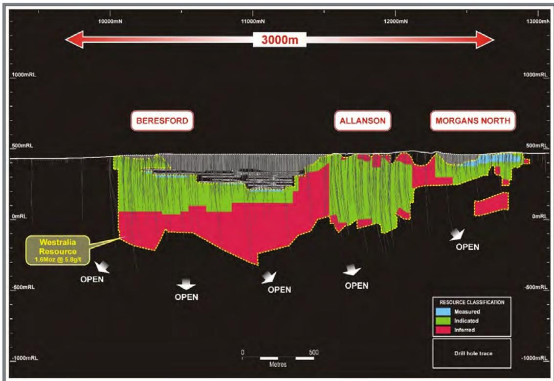
**Figure 6:** Longitudinal section of the 1.6 Moz Westralia Deposit showing the distribution of Measured, Indicated and Inferred Mineral Resources.
